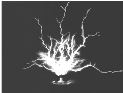
Miniature lightning bolts two feet long crackle from the Table Top Tesla Coil's discharge electrode.
