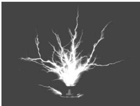
Miniature lightning bolts two feet long crackle from the Table Top Tesla Coil's discharge electrode.
